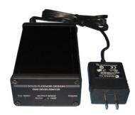
The *DMX DECELERATOR* is a DMX512 isolator and re-timing device. It can receive any signal within the DMX512 specification and it can accept some signals outside of the specification. It produces a DMX output signal with "relaxed" timing characteristics which are required by some DMX receiving devices.
