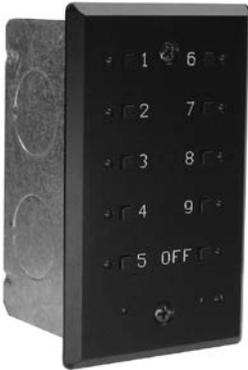
The Preset 10 Architectural is a lighting control station capable of storing up to ten presets. These presets are recorded by capturing the output of a DMX512 console. Each preset can then be assigned a unique fade time, from 0 to 999 seconds. Presets are recalled by pressing one of the buttons.
