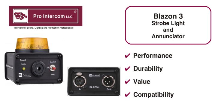
**Performance:** Blazon 3 is triggered by the same voltage which lights the normal signal lamps in the intercom system. Whenever any signal lamp button on any station in the same circuit is pressed, the Blazon/3 will be activated. The xenon lamp is permanently connected. The audible annunciator may be switched among constant, pulsed, and off. Circuitry is provided to sustain the Blazon 3 for 4 seconds after being triggered. The xenon lamp has a flash rate of 2Hz, providing 8 flashes per cycle.
