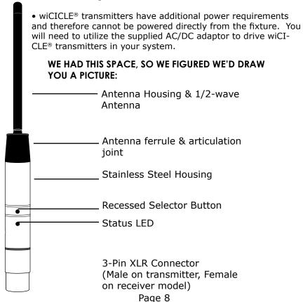
Each wiCICLE® acts as both a transmitter and a receiver, depending on whether a DMX source is applied to the integral XLR connector. This is an extremely powerful feature of the system, however, it also requires 1 piece of due dilligence, and that is the removal of extraneous DMX signals from your lighting rig BEFORE proceeding.
