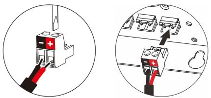
DarkFX Strip 1020 is wired to output terminal of DarkFX Drive 4 MKII. Each output terminal
