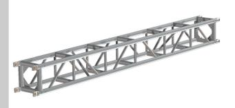
Applied Electronics Heavy Duty 12" Box Truss is manufactured with schedule 40, 1.9" OD x 0.145" wall main chords and 1.05" OD x 0.125" wall diagonal bracing. All components are 6061-T6 aluminum tubing and 5/8" grade 8 bolts are included for assembly of the truss elements. Heavy Duty 12" truss, combined with the matching corner blocks, can be used to construct a grid.
