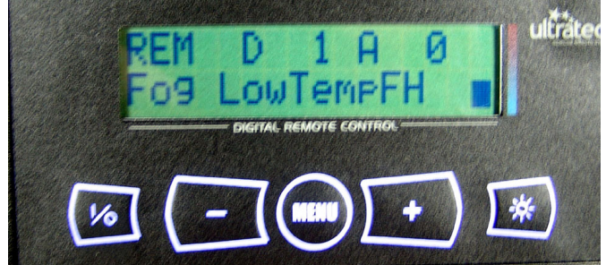
Note error from trying to turn on machine that is not yet hot enough.
