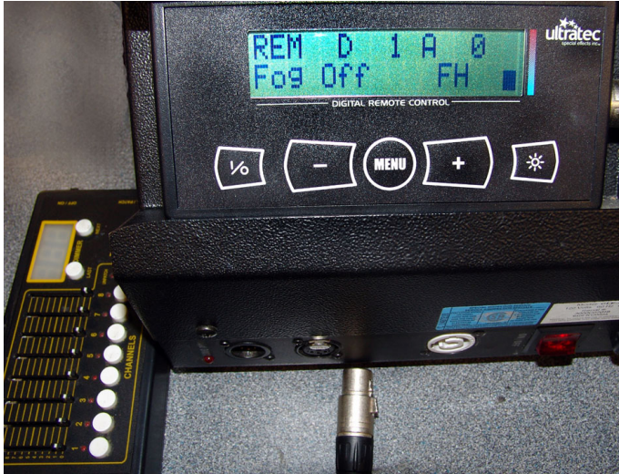
Machine turned on warming up with no DMX input. Note temperature bar graph shows low, Heater "H" is on and fog is turned off DMX is unplugged and DMX LED (bottom left) is not on.
