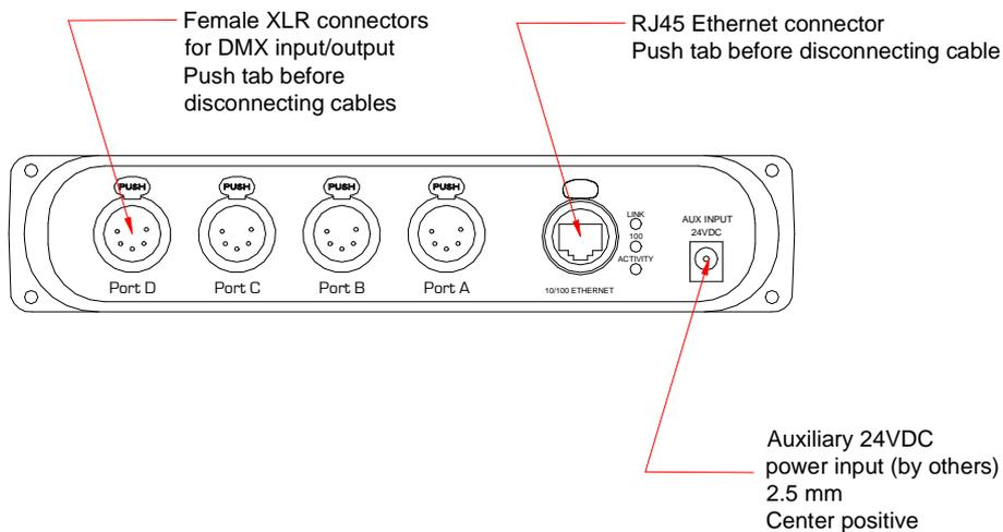
Pathport Quattros are available with female 5-pin XLR, female 3-pin XLR, RJ45 EtherCon and terminal strip connections for the DMX ports.
