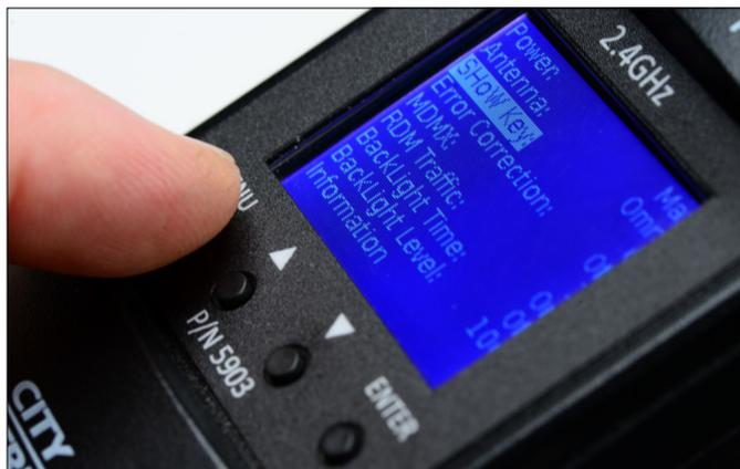
Setting SHoW IDs is simple using the Multiverse Node's four buttons and backlit LED display.
