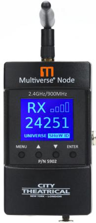
The **Multiverse® Node** is the first building block of the Multiverse system. Each **Multiverse Node** is a transceiver.
