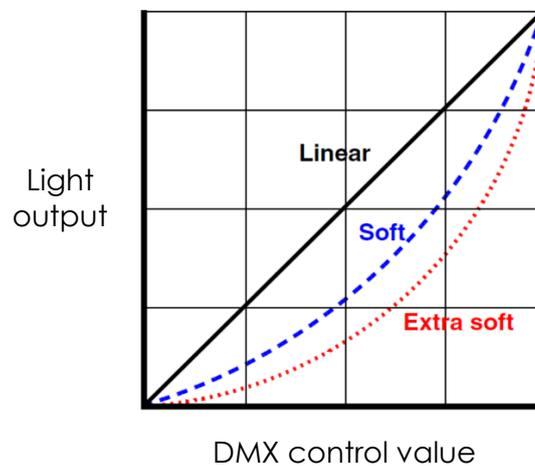
**Figure 3. Dimming curves**
