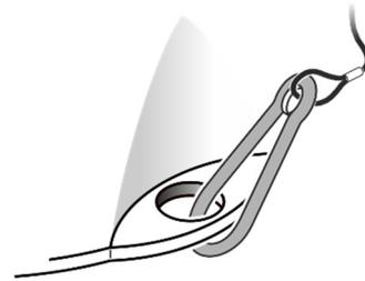
**Figure 6. Safety cable attachment**
