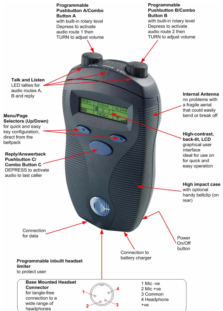
Figure 6-1: Overview of Beltpack Functions
