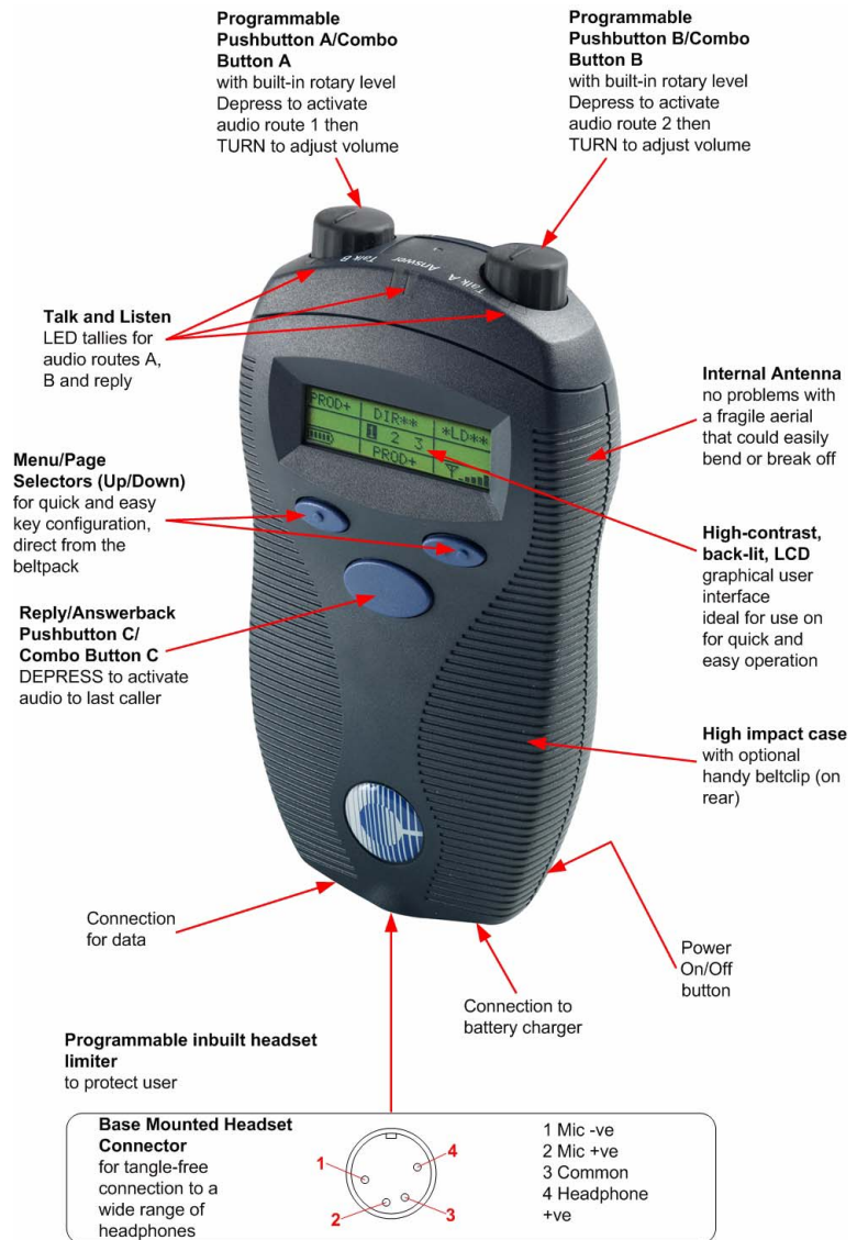
Figure 2-3: Overview of Beltpack Operation
