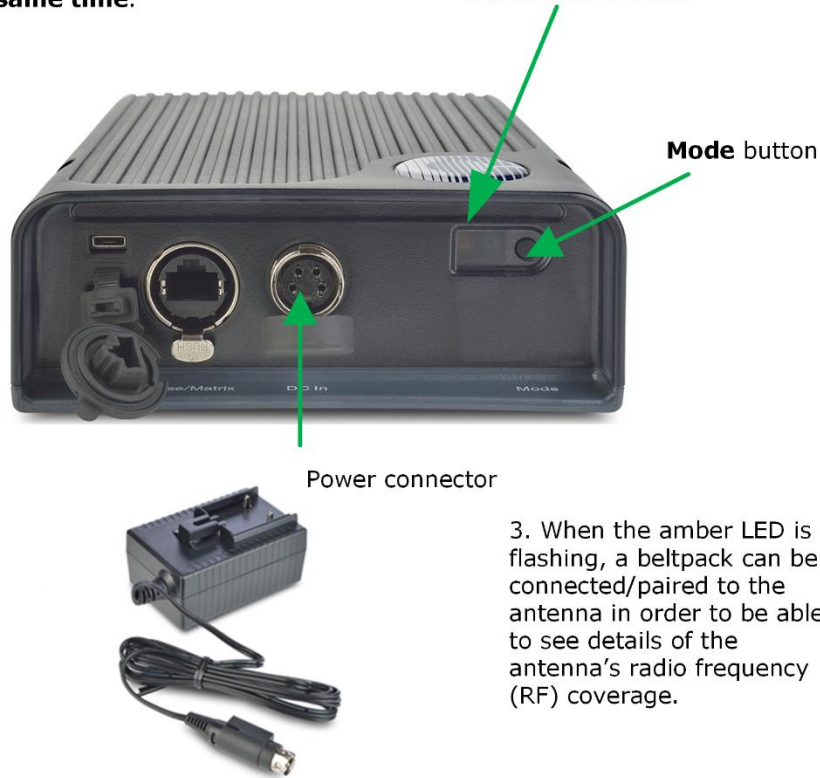
Figure 3-6 Using an antenna and beltack in standalone mode
