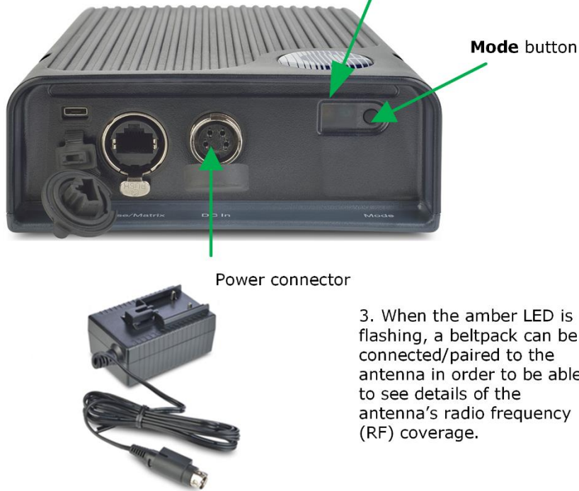
Figure 3-6 Using an antenna and belt-pack in standalone mode
