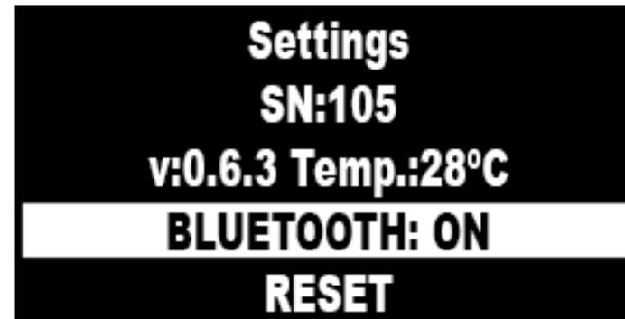
The Settings screen provides status information about the DMG DASH, including the serial number of the unit and the fixture's current operating temperature.
