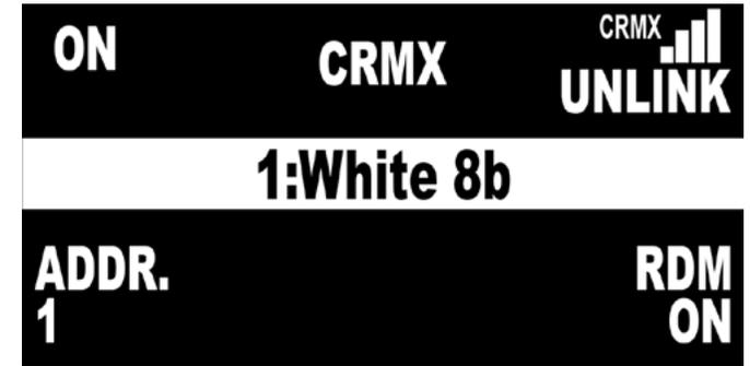
Use the Dimming & Selection Wheel to select the desired DMX profile.
