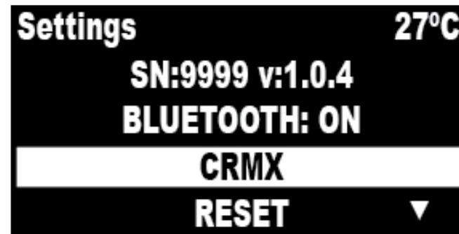
Press the Navigation Button or rotate the Dimming & Selection Wheel to highlight the CRMX option.
